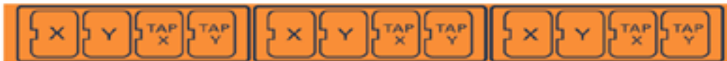
Figure 13 Port Label for G-TAP M451, M451T, M453T, M471, M471T, M471-SR10, and M473T
