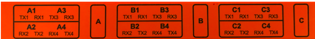
Figure 18 Port Label for Breakout Panels PNL-M341, PNL-M341T, PNL-M343, and PNL-M343T
